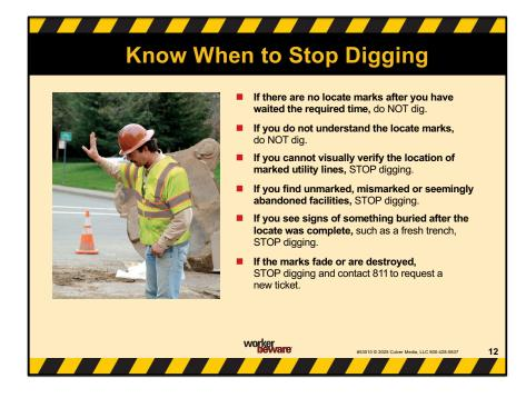
When you work around buried power lines and natural gas pipelines, knowing when to stop a job could save your life.
